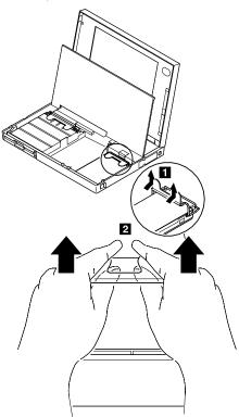
After replacing the hard disk drive, latch the removal strap into the correct position.
